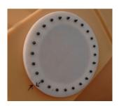
Assmann offers manway covers specifically designed to help minimize HCL fumes. Our bolted and gasketed manway covers are available in 16", 22", and 24" sizes depending on tank model. These covers include chemical resistant bolts that compress an XLPE foam gasket between the tank wall and a rigid cover. These manways should be used on any application where fumes need to be restricted from leaving the storage tank.
