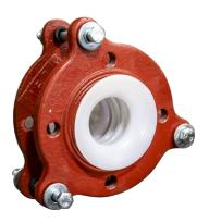
Flexible hoses or expansion joints must be used on all lower ½ sidewall connections. A lightweight isolation valve is permitted prior to the flexible joint. All piping must be supported independent of tank. Pipe supports must be installed after the flexible joint to allow the tank to expand and contract under normal service conditions. Polyethylene tanks expand and contract both laterally and vertically; expansion hose or joint must accommodate this expansion.
