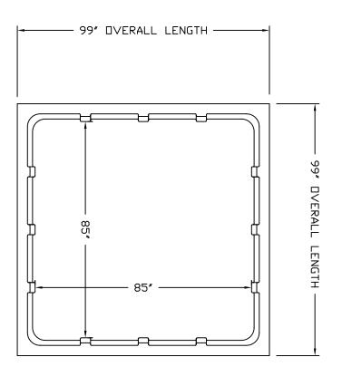
NOTES: 1. RESIN: LINEAR MEDIUM DENSITY POLYETHYLENE 2. CALCULATED CAPACITY: 1650 GAL.
