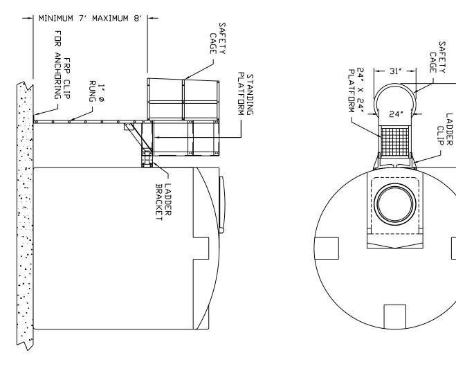
Polyethylene tanks are extremely slippery. Assmann does not recommend that anyone climbs or stands on the roof of a polyethylene tank. Unless special ordered, our ladders terminate purposely 48" below the tank roof, to prevent access to the tanks dome.
