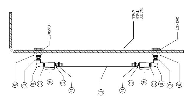
좆 C ₩ QTY SIZE 3/4" 3/4" 3/4" 3/4" 3/4" 1"I.D. 1/2 PVC SCH. 80 BULKHEAD FITTING W/ EPDM (STANDARD) PVC SCH. 80 BALL VALVE W/ EPDM (STANDARD) PVC SCH. 80 THREADED NIPPLES (STANDARD) PVC SCH. 80 90° ELBOWS (STANDARD) **ACCESSORIES** PP MALE THRD X HOSE BARB CLEAR FLEXIBLE PVC HOSE STAINLESS HOSE CLAMPS DESCRIPTION
