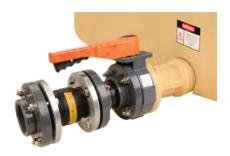
Flexible hoses or expansion joints must be used on all lower ½ sidewall connections. A lightweight isolation valve is permitted prior to the flexible joint. All piping must be supported independent of tank. Pipe supports must be installed after the flexible joint to allow the tank to expand and contract under normal service conditions. Polyethylene tanks expand and contract both laterally and vertically; expansion hose or joint must accommodate this expansion.
