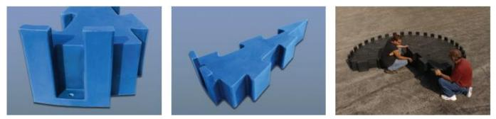
Assmann Corporation will ship the modular tank stand on multiple skids. You need to select a suitable flat-level surface that can support the weight of the tank, stand, and chemical being stored. Start by placing the pie-shaped pieces with the molded-in edge facing upward. Two people can easily lift the interlocking pieces and slide them together as shown.
