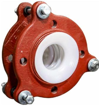
**Flexible hoses or Expansion Joints must be used on all lower ½ sidewall connections.** A lightweight isolation valve is permitted prior to the flexible joint. All piping must be supported independent of tank. Pipe supports must be installed after the flexible joint, to allow the tank to expand and contract under normal service conditions. Polyethylene tanks expand and contract both laterally and vertically; expansion hose or joint must accommodate for this expansion.
